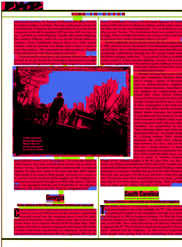
Figure 3. An example of visual presentation of results at the page level. Ground truth is in medium-dark (blue) colour while segmentation regions are in lighter (light green) colour. Overlapping regions are in darker (red) colour. Split and merged regions can be seen at a glance.
