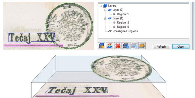
Figure 7. Layers: top-left: Stamp over text and separator; top right: Layer dialogue; bottom: Illustration of layers.
